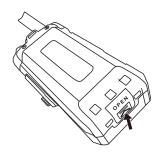
To remove the battery pack, make sure the transceiver has been turned off, and then press the battery released latch in the bottom of transceiver, and pull the bottom part of battery away from the transceiver body, and remove the battery.
