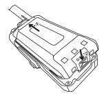
Insert the top part of the battery pack into the top 2 slots of the transceiver and then press the battery pack down until a "click" sound is heard.
