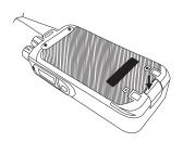
To remove the battery pack, make sure the transceiver has been turned off, and then open the bottom's buckle, Remove the battery when the batter pops up
